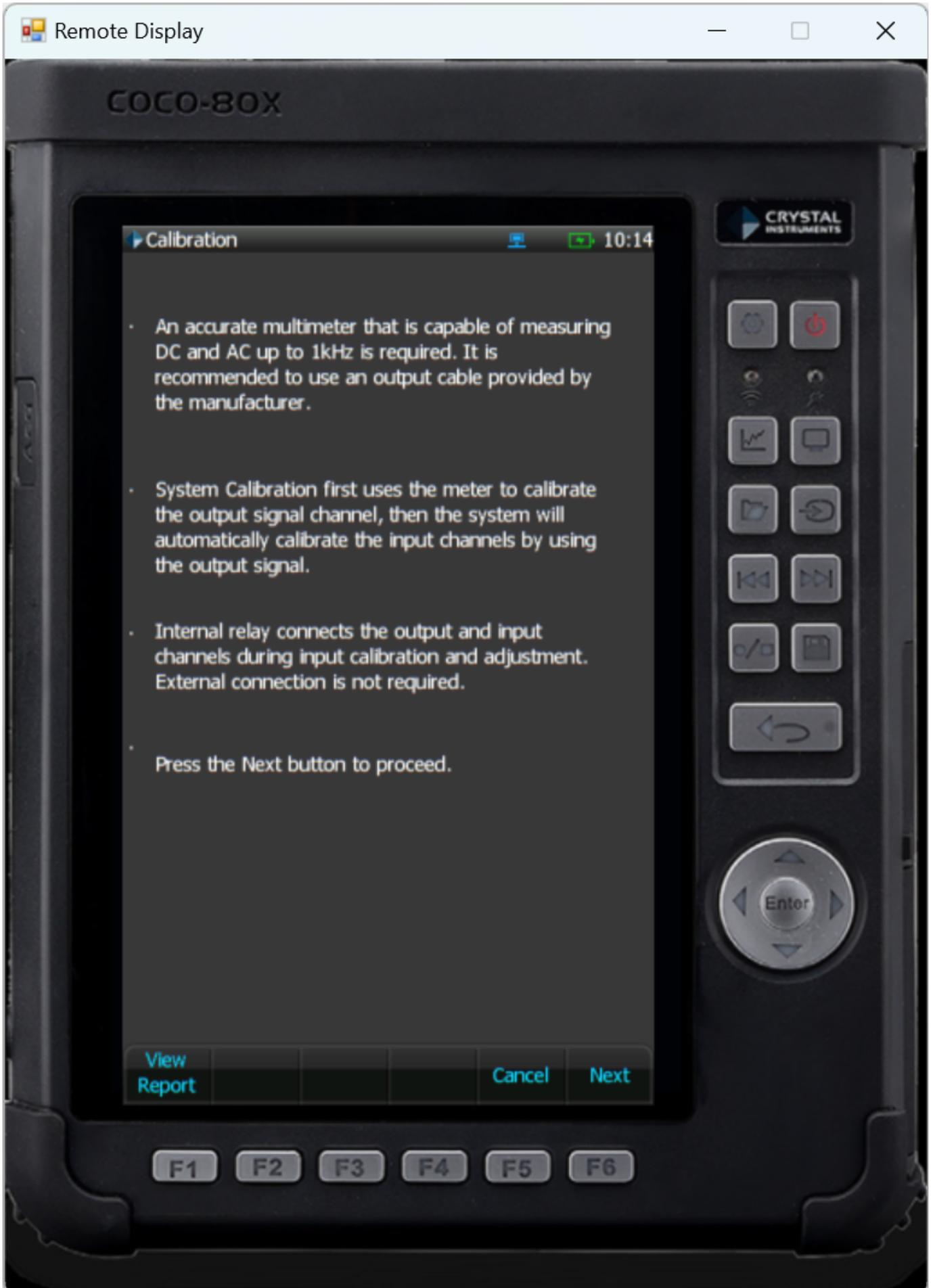
Connect the CoCo output to the multimeter. The CoCo will then give instructions on how to perform the calibration. The operator will need to enter the multimeter readings into the CoCo.
