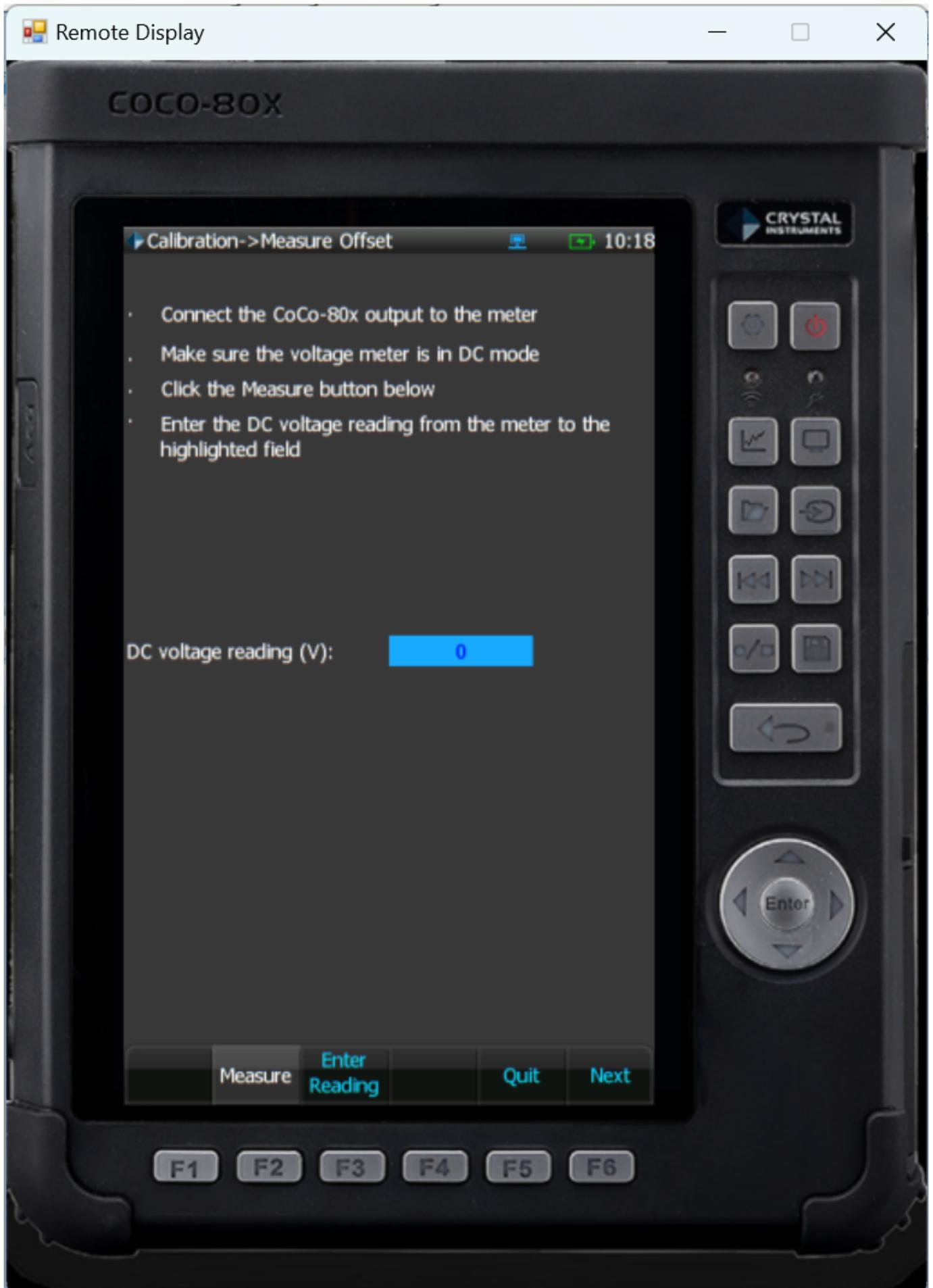
Keep following the on-screen instructions. Both AC and DC measurements will be taken. After all measurements have been entered, the CoCo will validate the input channels. After this a window will
