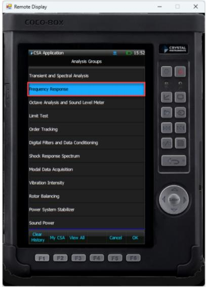
• Select the test that you wish to run. On this screen you can see important parameters like *Channels Enabled, Max Sampling Rate,* and a description of the test.
