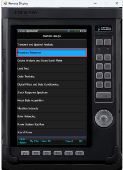
• Select the test that you wish to run. On this screen you can see important parameters like *Channels Enabled, Max Sampling Rate,* and a description of the test.
