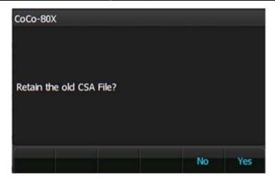
Press "Yes" (or "keep" on recent versions) to keep all CSA settings the same, or press "No" (or "Reset" on newer versions) to reset all CSA settings to the default configuration. It will have no effect on saved signal data.
