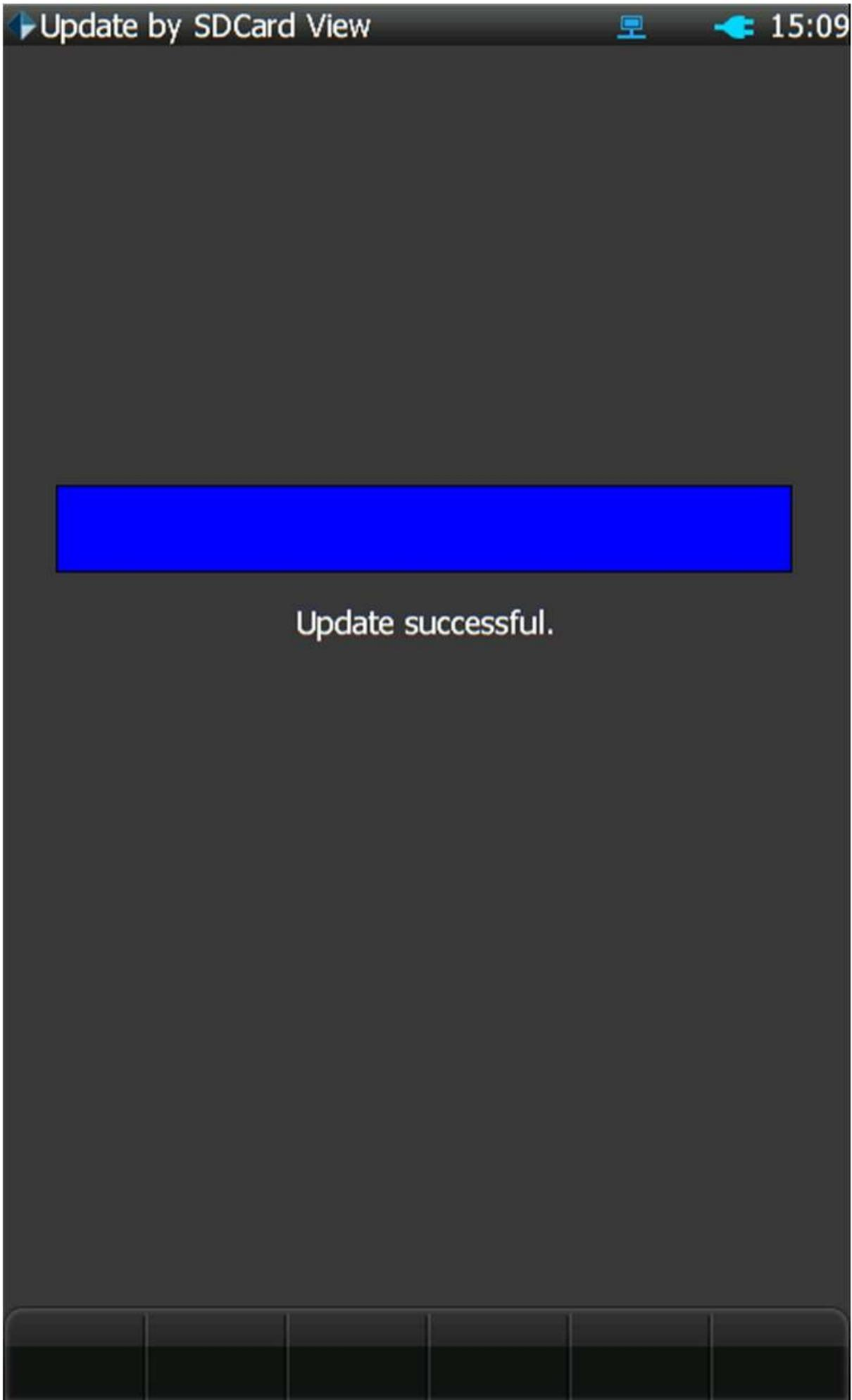
The device will shut down once the update is finished. To verify that the correct software version was installed, press **Setup**  $\square$  **F2 (About)**. To check the software options, press **Setup**  $\rightarrow$  **F2 (About)**  $\rightarrow$  **F1 (Software Options)**.
