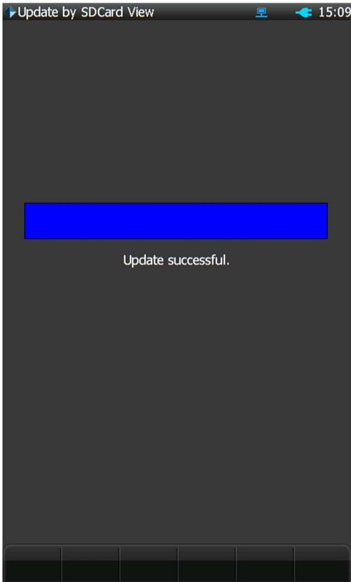
The device will shut down once the update is finished. To verify that the correct software version was installed, press **Setup** → **F2 (About)**. To check the software options, press **Setup** → **F2 (About)** → **F1 (Software Options)**.
