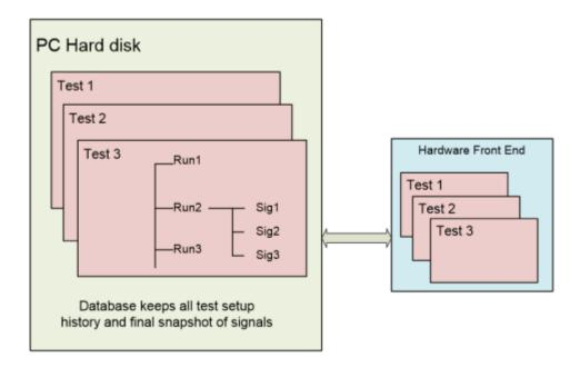
On the PC, the database keeps all the history, testing setup, and the final snapshot of measured signals. If you want to back up the setup of ALL tests, simply back up or export the complete database.
