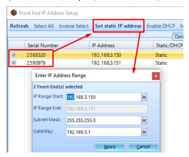
Select the module(s) and click **Set static IP address**. Fill in the IP address(es), subnet mask, and gateway as needed. The LED on the Spider will flash for a couple seconds, indicating that the new IP
