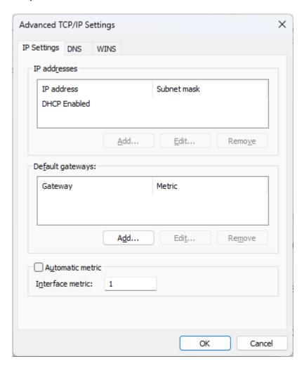
Right-click on the Spider network adapter, go to **Properties > select "Internet Protocol Version 4 (TCP/IPv4)" > Properties > Advanced**, uncheck **Automatic metric** and set **Interface metric** to 1 (lower is higher priority)
