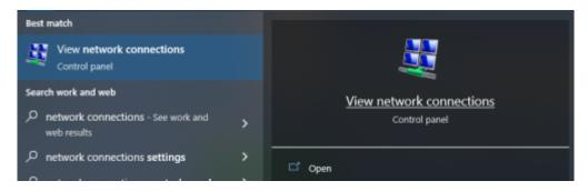
Right-click on the Ethernet connection to the Spider, click "Properties". Then, select "Internet Protocol Version 4 (TCP/IPv4)" and click "Properties". Then, select "Use the following IP address:" and enter in the desired static IP address values.
