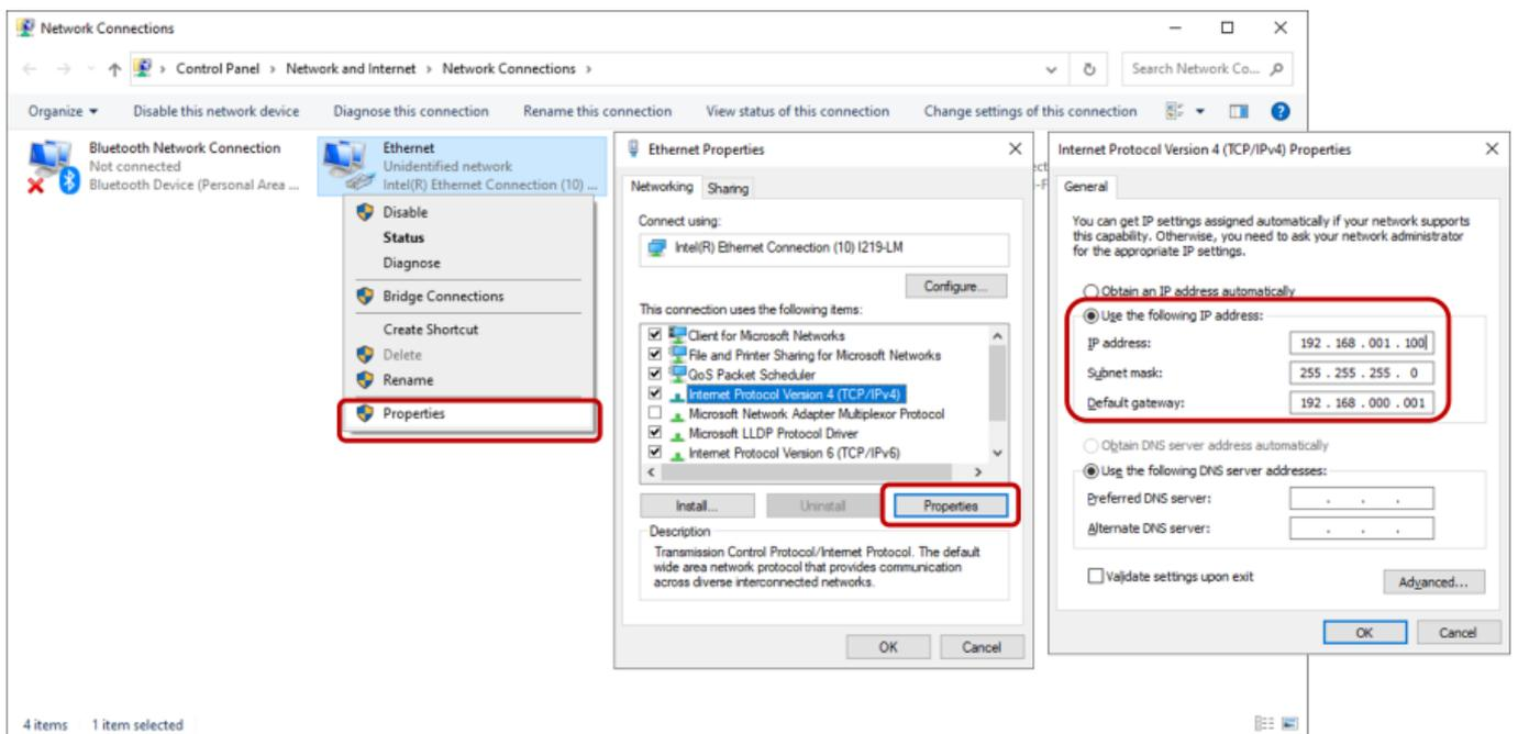
The PC IP address, Spider IP address, and gateway should all share the first three numbers, while having a unique fourth number. The subnet mask should be “255.255.255.0”.
