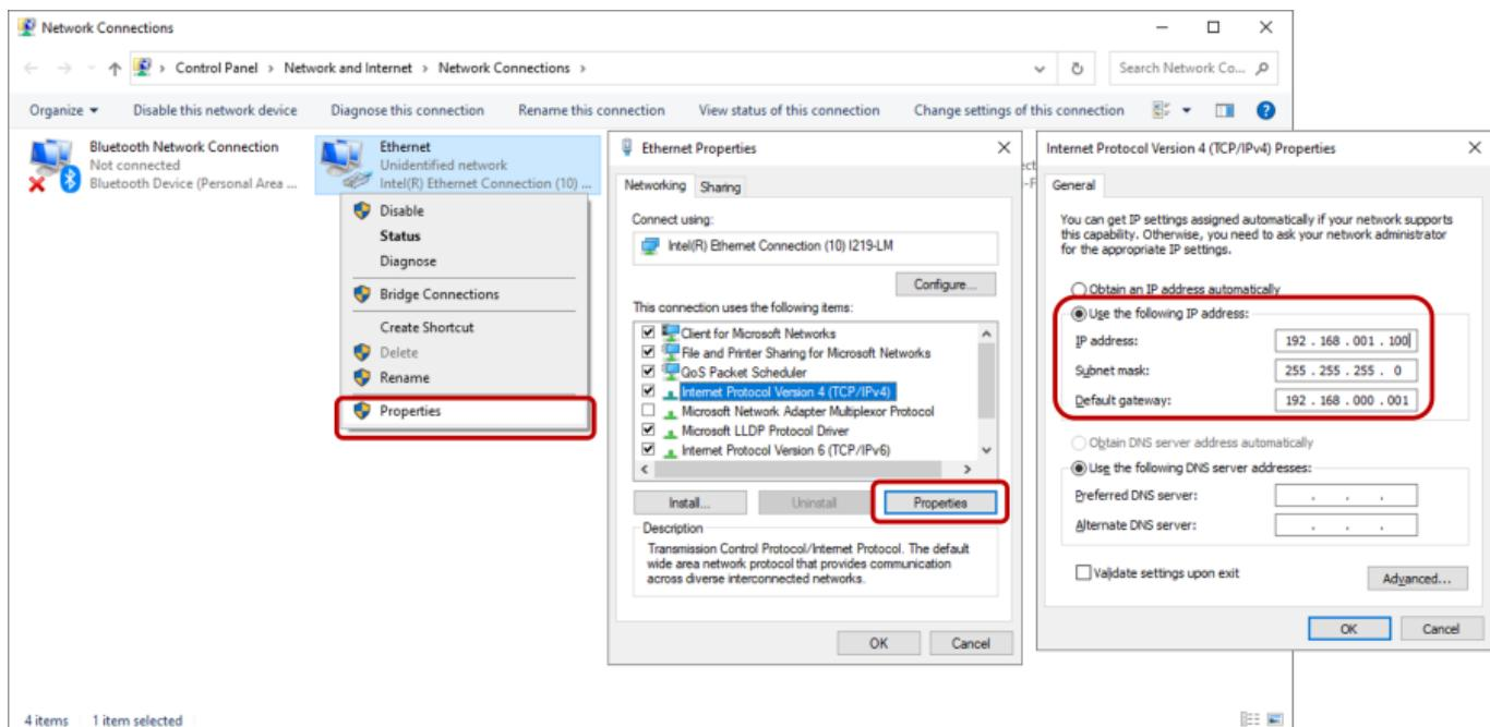
The PC IP address, Spider IP address, and gateway should all share the first three numbers, while having a unique fourth number. The subnet mask should be “255.255.255.0”.
