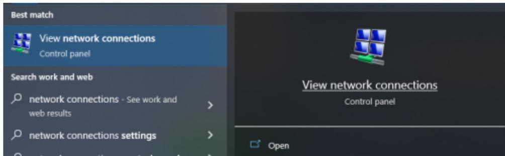
Right-click on the Ethernet connection to the Spider, click “Properties”. Then, select “Internet Protocol Version 4 (TCP/IPv4)” and click “Properties”. Then, select “Use the following IP address:” and enter in the desired static IP address values.
