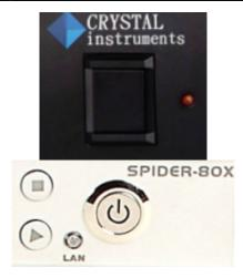
Warning: Never press this button to turn the power off while the controller is running. In the case of emergency, press the Stop button on the front, or use the Abort contact switch connected to the back.
