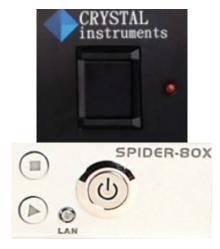
Warning: Never press this button to turn the power off while the controller is running. In the case of emergency, press the Stop button on the front, or use the Abort contact switch connected to the back.
