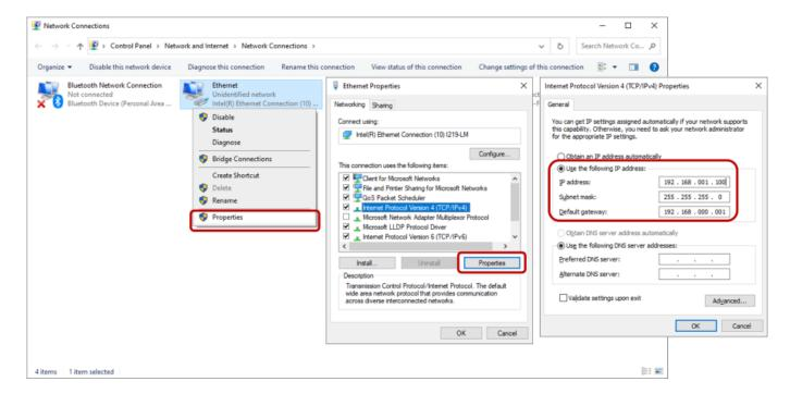
The PC IP address, Spider IP address, and gateway should all share the first three numbers, while having a unique fourth number. The subnet mask should be "255.255.25.0".
