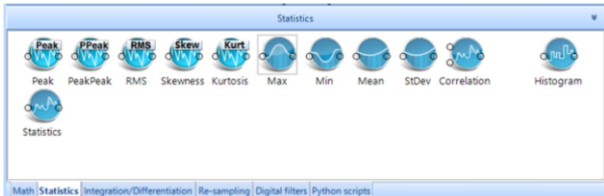
Statistics supports a variety of functions used in data interpretation. Including several common functions i.e. Min, Max, Mean. It also supports more specialized operations: Peak to Peak operator saves the greatest displacement between signal minimum and maximum of oscillation during time block. RMS calculates the effective signal strength over a period.
