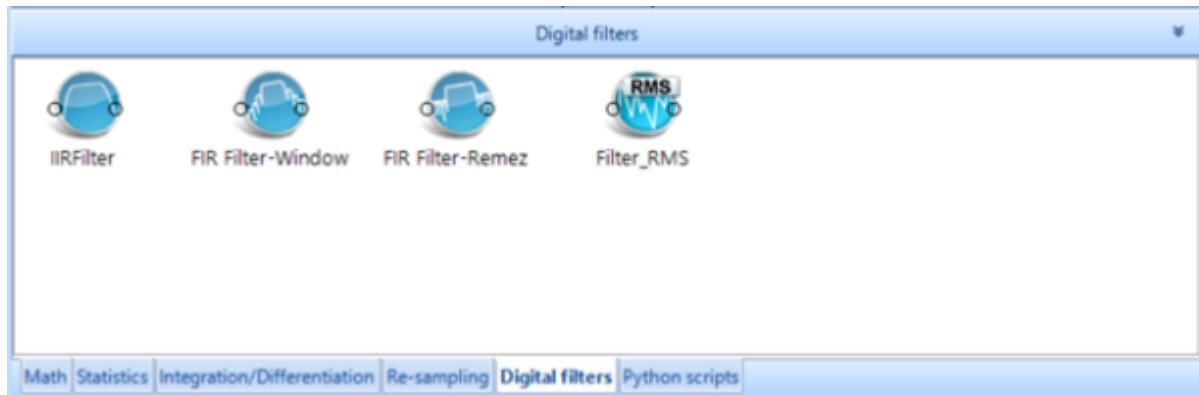
Finite Impulse Response filters: Have a set time duration of response. FIR filters do not have a feedback loop and feature a constant group delay. This means that an input signal will have a uniformly delayed output and will have no distortion. FIR filters are defined by:
