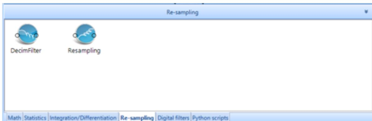
DecimFilter the decimator filter reduces the amount of time domain point to make computing more efficient. The data is put through a low pass anti-alias filter and then every nth point is kept. Resampling filter updates the sample to be L/M. The input time stream data is up sampled by L, there are L-1 data points filled in with zeros between time stream data input points. Next, Low pass anti-aliasing filter is applied. Finally, the data is downsampled by M. Every Mth point is kept.
