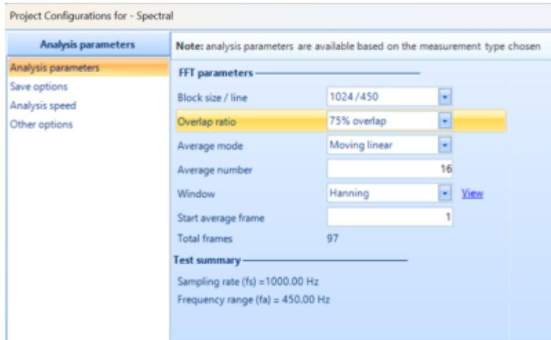
Make selections for block size / spectral lines to determine  $\Delta f$  and dynamic range. Overlap ratio, recommended at least 50% for Hanning window. Average mode and average number based on testing requirements. Window selection can be left as Hanning for most testing applications; Uniform may be desired for shock or transient impulse testing.
