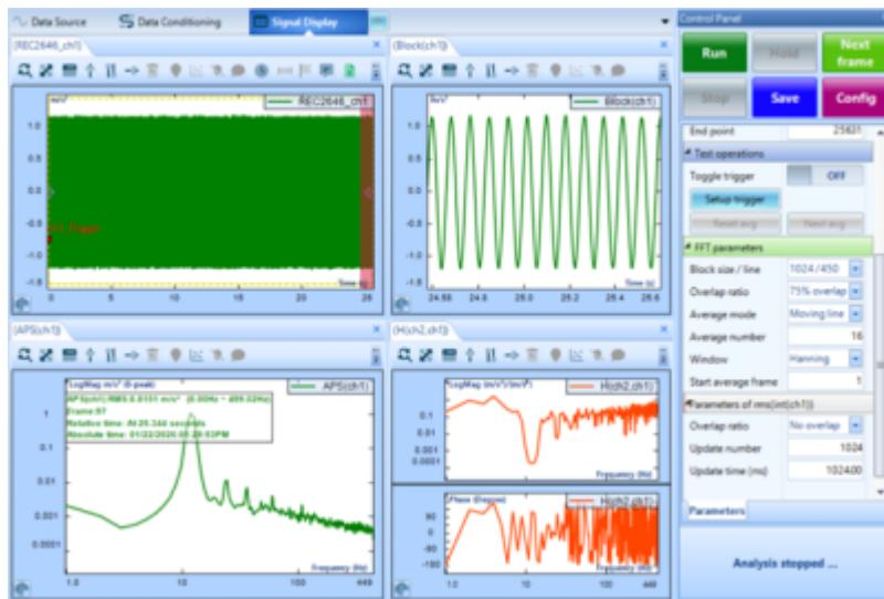
Once setup is complete select Run from the control panel in the upper right of the screen. Processed data will display in windows and be saved to signal folders as the signal is run in real time. Save option in Control Panel will become available to user.
