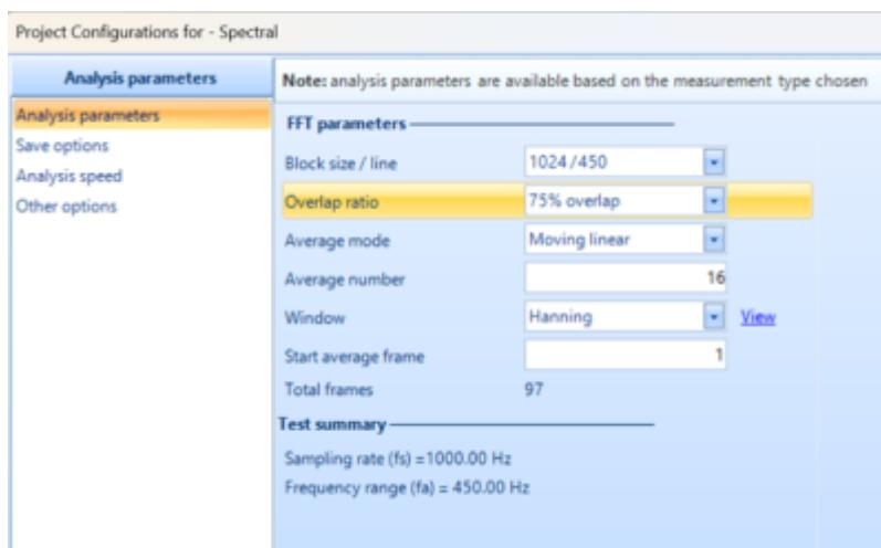
Make selections for block size / spectral lines to determine  $\Delta f$  and dynamic range. Overlap ratio, recommended at least 50% for Hanning window. Average mode and average number based on testing requirements. Window selection can be left as Hanning for most testing applications; Uniform may be desired for shock or transient impulse testing.
