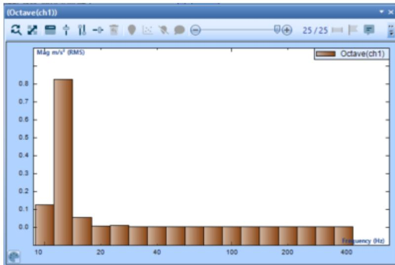
Octaves are defined as a doubling of magnitude. Moving a single octave can move from a frequency of 4 Hz to 8 Hz or 1000 Hz to 2000 Hz. Octave analysis often breaks Octaves into bins  $1/N$  times. Octave filter displays responses in frequency bins. Passband filters are applied to time stream data and the resulting magnitude of frequencies are overlaid into single response to show strength of signal by frequency octave.
