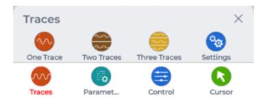
Tapping on any of the numbered trace button will change how many traces are displayed.
