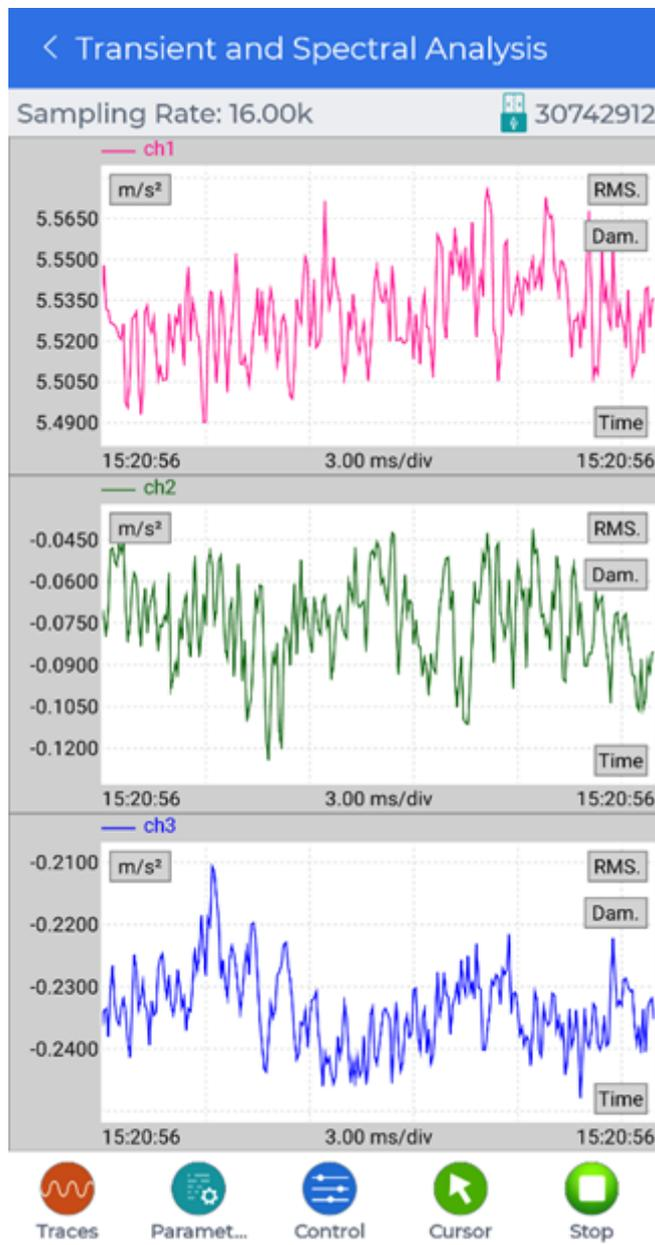
To edit any recording settings, tap the **Parameters** button to open a menu and **slide to the left** to reveal the **Record Setup** button. Tap on the **Record Setup** button to edit what signals to record and how many points or how long to record.
