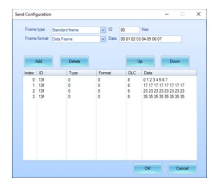
Frames of CAN bus data can be configured with the desired ID (in Hexadecimal) and Data body.
