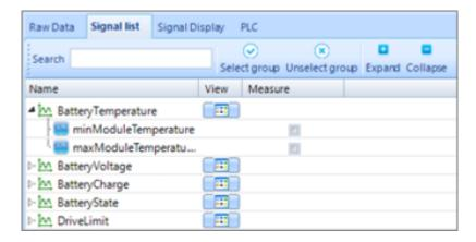
Filter through the signals in your DBC file using the Search box above. Click on the **View** icon to see more details about the configured CAN bus entry. Enable the **Measure** checkbox to enable it in the
