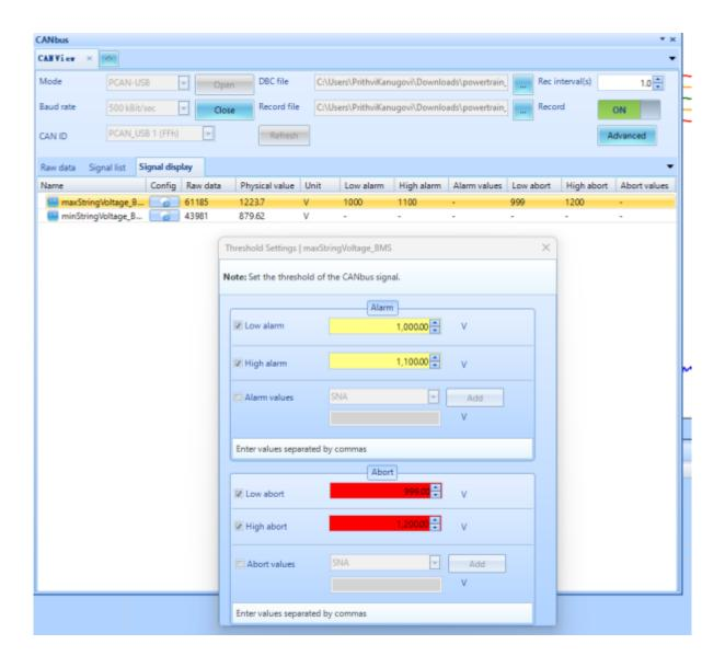
Click on the **Config** icon for each given entry to configure the Alarm / Abort thresholds.
