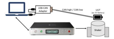
To read CAN bus signals from the UUT, first connect the CAN Bus USB adapter to the PC running EDM. On the other end of the CAN bus adapter, use the screw terminals to connect the CAN high (CANH)
