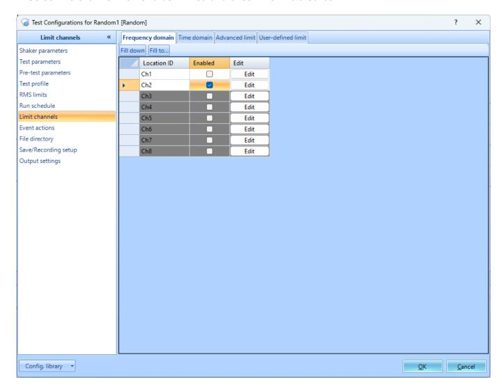
3. A limit profile window will open. Specific High Abort and High Alarm limits can be set up.
