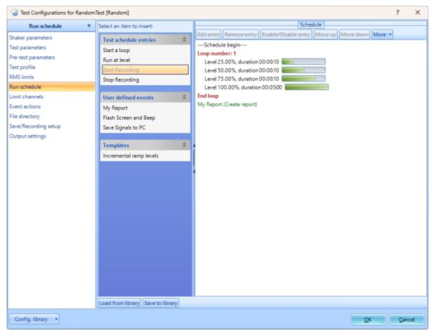
Start a loop: Adds a new loop to the schedule – EDM will open a prompt for how many times to loop. Double-click on an existing loop number to edit the number of times for that entry.
