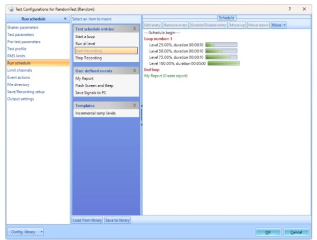
Start a loop: Adds a new loop to the schedule – EDM will open a prompt for how many times to loop. Double-click on an existing loop number to edit the number of times for that entry.
