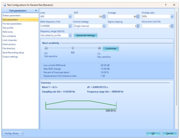
Lines: The useful number of spectral lines, proportional to block size. Increasing the lines / block size will improve the resolution of the frequency spectrum (allowing better detection of lower frequencies) at the tradeoff of increased calculation time and slower response.
