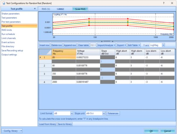
Breakpoint Table: Breakpoints can be added via **Insert row**, **Delete row** and **Append row**. Use **Clear table** to clear out all rows except for the first and last row. Breakpoint Calculation: In the profile editor, EDM can calculate the crossover point given a specified slope and point value. If a '?' is entered as a Frequency or Amplitude value, EDM will interpolate that value given the slope before and after that point.
