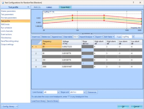
Breakpoint Table: Breakpoints can be added via **Insert row**, **Delete row** and **Append row**. Use **Clear table** to clear out all rows except for the first and last row. Breakpoint Calculation: In the profile editor, EDM can calculate the crossover point given a specified slope and point value. If a '?' is entered as a Frequency or Amplitude value, EDM will interpolate that value given the slope before and after that point.
