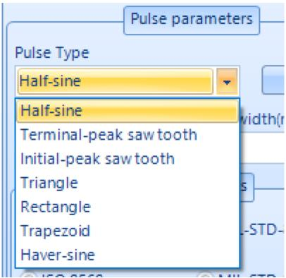
Amplitude/Width: Amplitude sets the peak acceleration value of the pulse. Pulse width sets the width of the pulse in milliseconds. Narrower pulses have greater high-frequency components.
