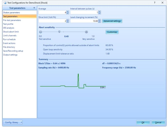
Interval Between Pulses: The time period between successive pulses. The value should be large enough for the system's response to dampen out after a pulse. It is effective when it is larger than block time.
