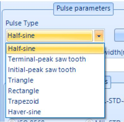
Amplitude/Width: Amplitude sets the peak acceleration value of the pulse. Pulse width sets the width of the pulse in milliseconds. Narrower pulses have greater high-frequency components.
