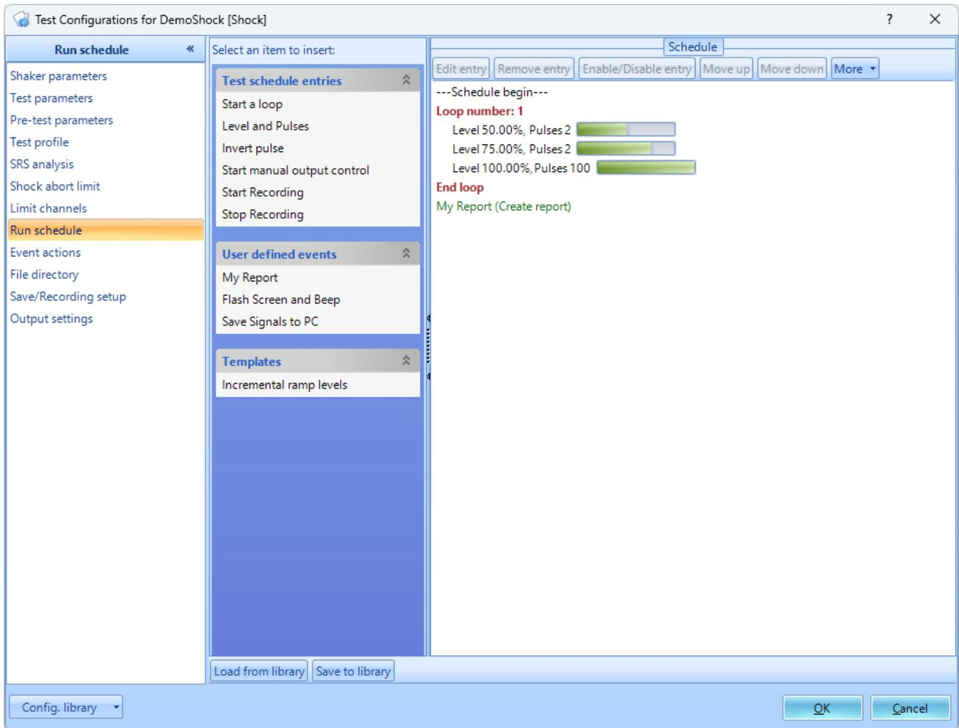
Level and Pulses: Level and Pulses output the set number of pulses at the set level, given in percent.
