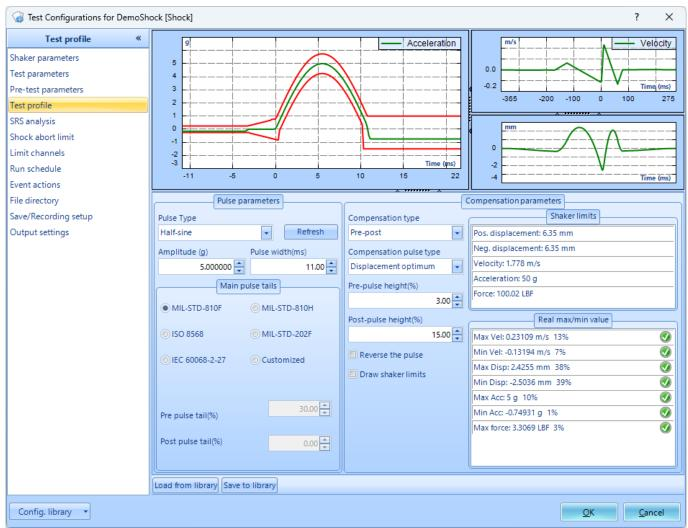
*Pulse Type*: Pulse Type is the shape of the main pulse. The options are half-sine, terminal-peak sawtooth, initial-peak sawtooth, triangle, rectangle, trapezoid, and haver-sine. The shapes have different frequency characteristics and are suitable for simulated different impulse conditions. Many testing standards specify the pulse shape to be used.
