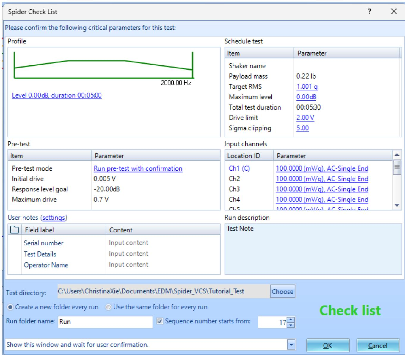
Run Schedule, Test Profile, Pre-test Parameters sections can all be found in the control panel clicking the **Config** button.
