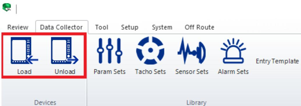
To upload using SD card, in VDS, click **Data Collector** > in the **Devices** menu, click **Load** > Click **File folder (Name is CoCo-80)** > Select the Device you are using > Select the card name > Click **Next** > Click the **Browse** button > select the proper path > **choose the folder CoCo-80** > Click **OK**.
