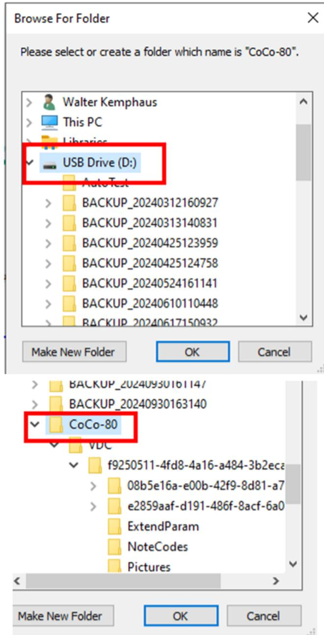
To upload using SD card, in VDS, click **Data Collector** > in the **Devices** menu, click **Load** > Click **File folder (Name is CoCo-80)** > **Select** the Device you are using > Select the card name > Click **Next** > Click the **Browse** button > select the proper path > **choose the folder CoCo-80** > Click **OK**.
